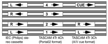
Notice that the stereo cassette arrangement allows you to use both sides of the cassette, by playing the tape in the other direction. The Porta02, however, uses the whole width of the tape. Notice also that
